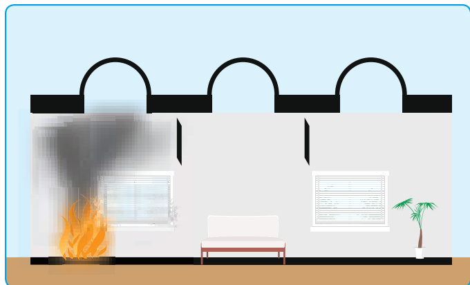
Principle of smoke ventilation (with skydomes).
